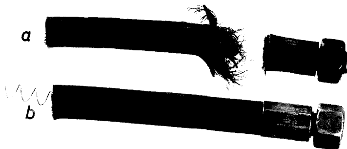
Fig. 6. End of rubber hose assembly DN12, type 4 SP with length L = 1500 mm ( p_{\text{burst, min}} = 1660 bar) after a test with decomposition of high pressure acetylene at an initial pressure of 26 bar. a Normal high pressure rubber hose assembly. b Same high pressure rubber hose assembly with a spiral inserted inside.
